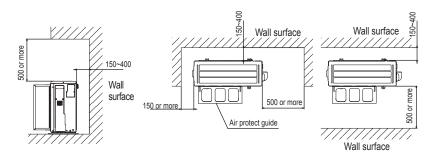
(2) Multiple unit installation: \*Installation of multiple units in series must be no more than five units.
